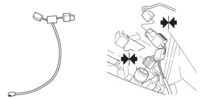
5. Plug the 6 position dual row connector from the supplied power harness into position # 4 on the controller
