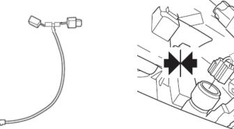
5. Plug the 2 position connector from the supplied power harness into position # 5 on the controller
